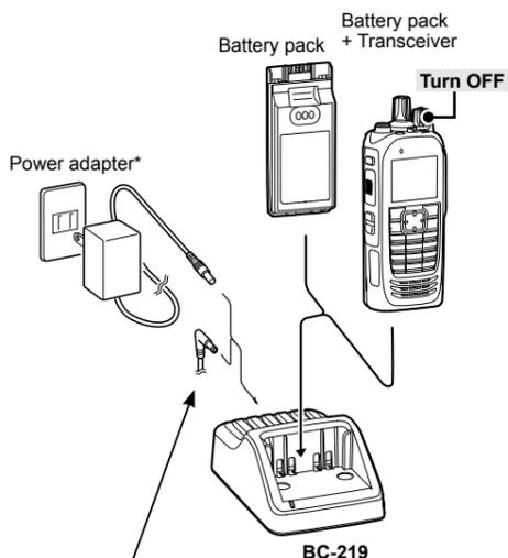
The OPC-515L\* (for a 13.8 V power source) or the CP-23L (for a 12 V cigarette lighter socket) can be used instead of the power adapter.
