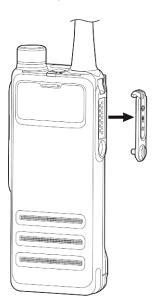
2. Insert the audio accessory plug into the accessory connector.
