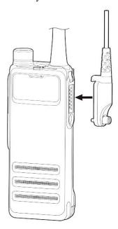
3. Tighten the screw on the audio accessory plug.
