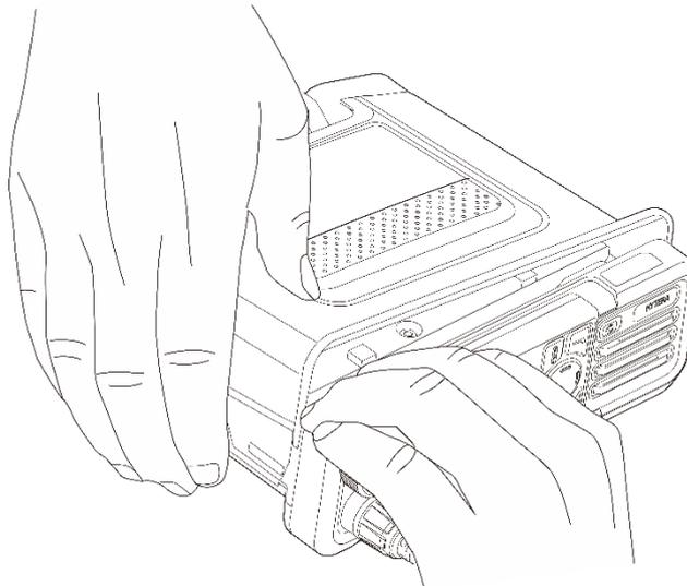
3. Insert the TF card to the metal card slot properly as directed in the following figure.
