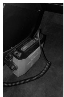
Mount radio bracket on a solid, steady surface Use suppled screws or bolts and nuts
