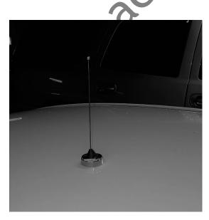
Attach antenna to the roof mount and snug with a crescent wrench
