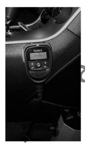
Mount the mic clip on a solid, steady surface that is easily accessible for the user
